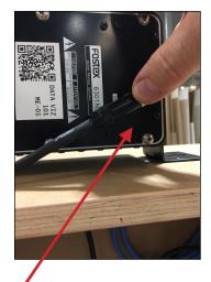
Pass power and audio cord through hole in top and connect to speaker.
